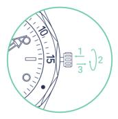
Please make sure that the crown is fully screwed in, otherwise water can enter the case and the water resistance is no longer guaranteed. To do this, push the crown in (1) and simultaneously turn it clockwise (2) until it is firmly seated on the case. To release the crown, turn the crown (3) counterclockwise.
