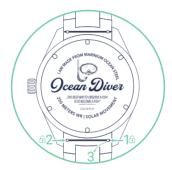
Press both bracelet locks inwards to unlock (1 & 2) and simultaneously move the bracelet away from the watch (3). Interchangeable bracelets can then be reattached in reverse order.
